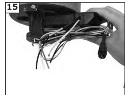
Slide remote receiver into mounting bracket.
